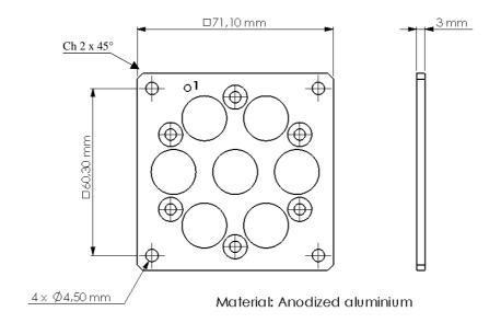
For R573 series, 3 to 6 positions with connectors 1.6/5.6, N, BNC, TNC
